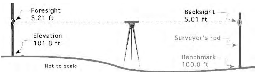
FIGURE 15.3. Foresight rod reading.
